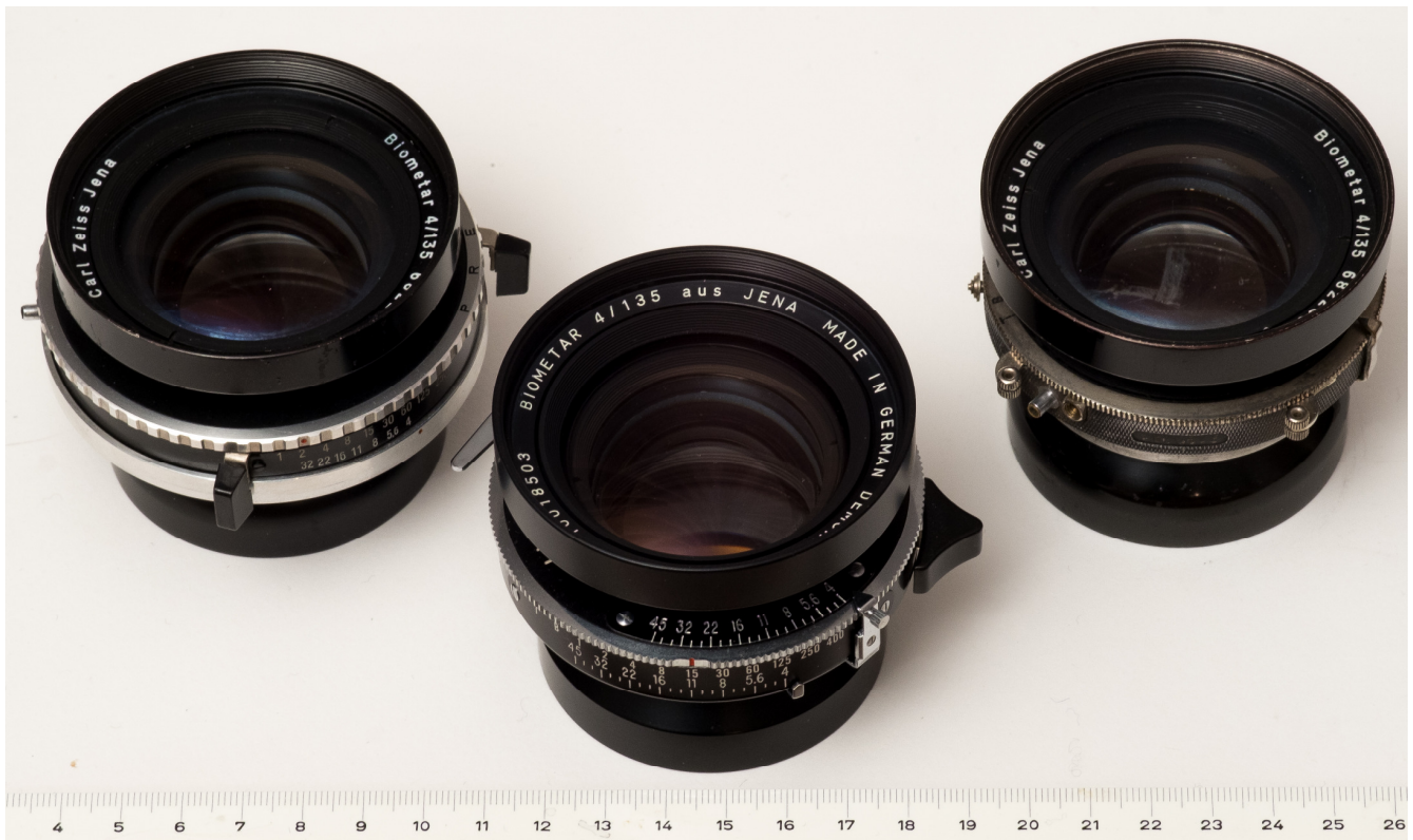
Fig. 8: Three versions of the Biomatar 135mm f/4. Back left: Original prototype version in Prestor 1 shutter. Back right: Original prototype version adapted in the GDR to a Western Synchro-Compur shutter. Front: Export version ("aus Jena") in older style Copal 1 shutter from the 1970's. Scale is in cm.
