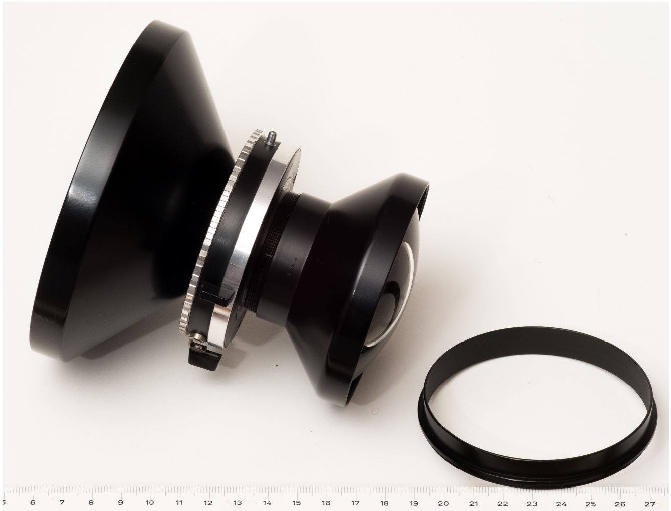
Fig. 7: Lamegon 90mm f/4.5 with the ring on the back lens cell removed. This ring, which protects the back lens element from mechanical damage, limits the coverage to about 92° by mechanical vignetting, instead of the 105° the lens is capable of. Scale is in cm.
