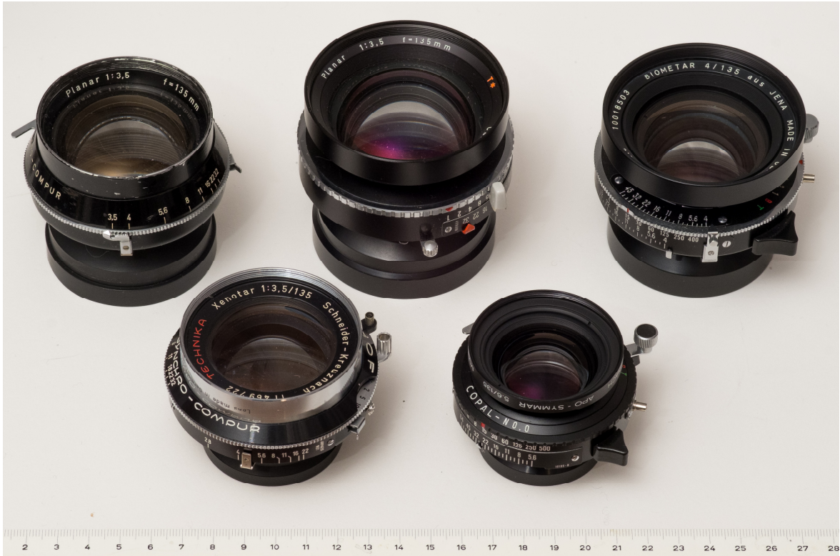
Fig. 9: The CZJ 135mm f/4 Biometar (top right) together with the Zeiss Oberkochen 135mm f/3.5 Planar from 1956 (top left) and the 1969 Planar redesign (top center), the Schneider 135mm f/3.5 Xenotar (front left,) and a 135mm f/5.6 Schneider Apo-Symmar (front right). Scale is in cm.
