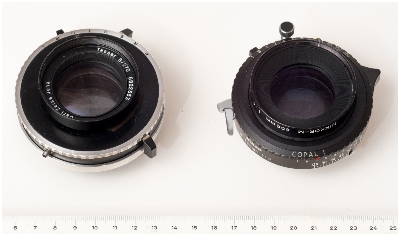
Fig. 11: Tessar 270mm f/8 in Prestor 1 shutter (left) together with Nikon M 300 f/9 in Copal 1 (right) for comparison. Scale is in cm.
