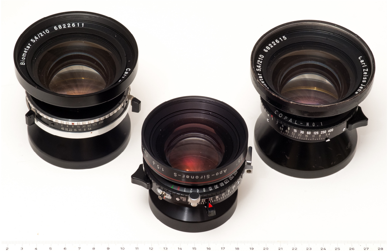
Fig. 10: Top left: Biometar 210mm f/5.4 in original Prestor 1 shutter. Top right: Biometar 210mm f/5.4 adapted to a modern Copal 1 shutter. Front: Rodenstock Apo-Sironar S 210mm f/5.6 for comparison. Scale is in cm.
